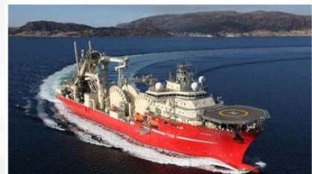
TechnicFMC "Deep Energy" Reel Lay vessel with 5,600T of pipe product storage capability
