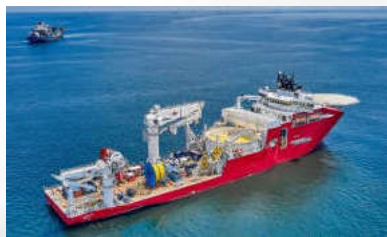
Aker "Connector" flexlay vessel with 7,000T of storage
