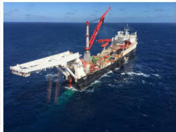
Alsea "Solitaire" S-Lay vessel with over 1,050T of pipe tension capacity and 22,000T of pipe storage
