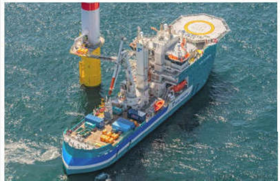
SOV transferring workers and equipment to offshore wind turbine
