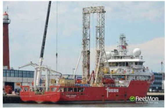
"Furgo Voyager" 270ft long DP2 vessel fitted with 10,000ft water depth heave compensated seabed coring tower
